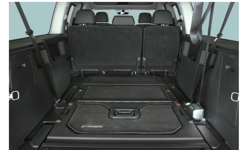
F-Style Lowered Floor Conversion with Genius Ramp on Volkswagen Caddy Maxi
