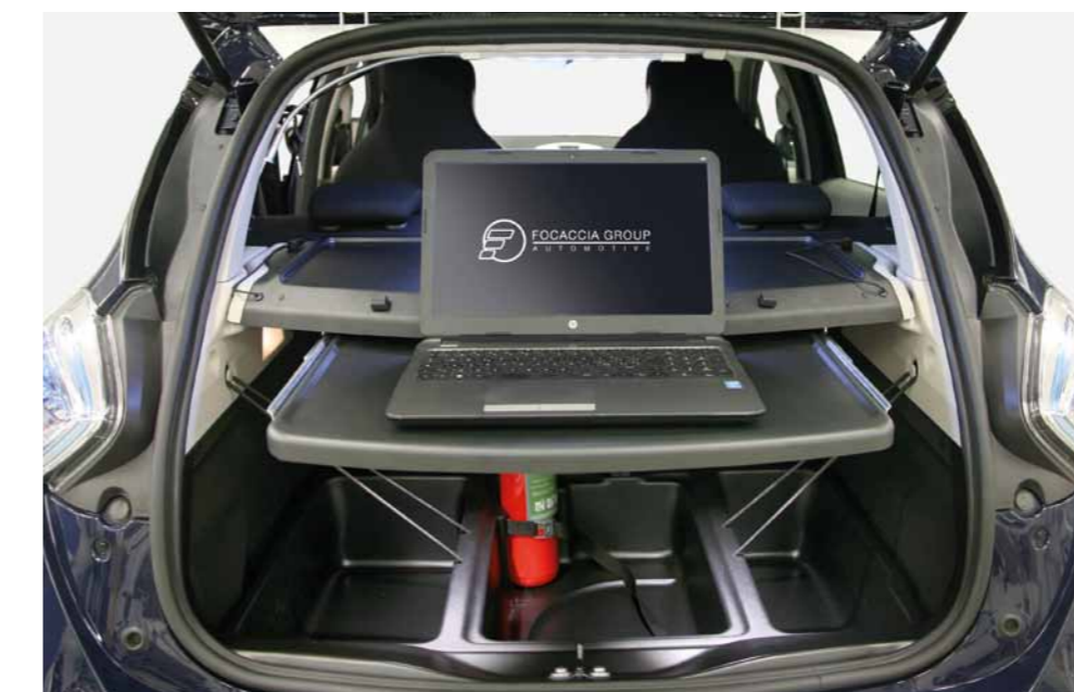
Thermoformed ABS Trunk Organizer with integrated writing desk replacing the original parcel shelf
