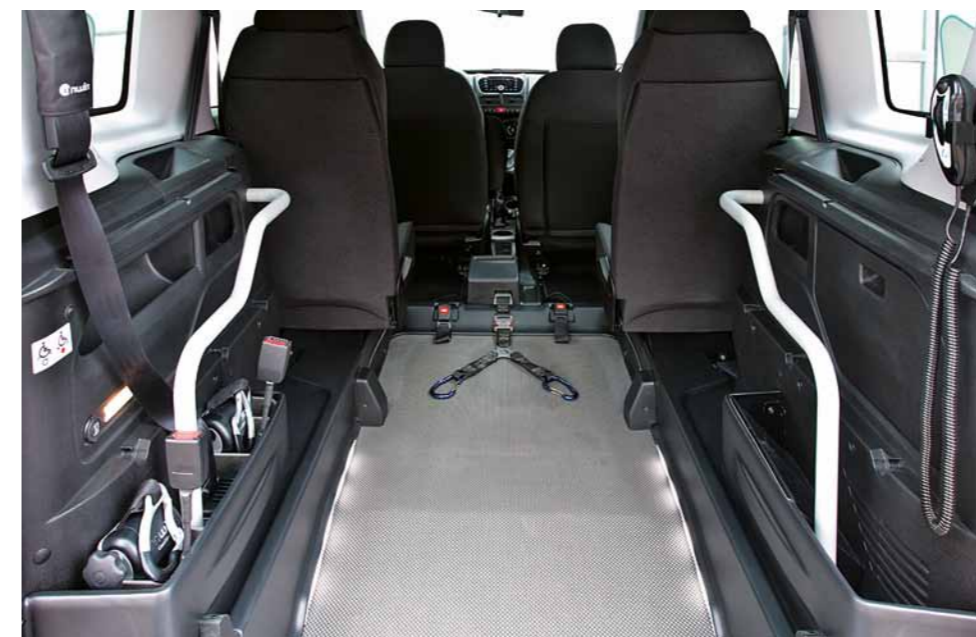
F-Style One Lowered Floor Conversion on Fiat Doblò
