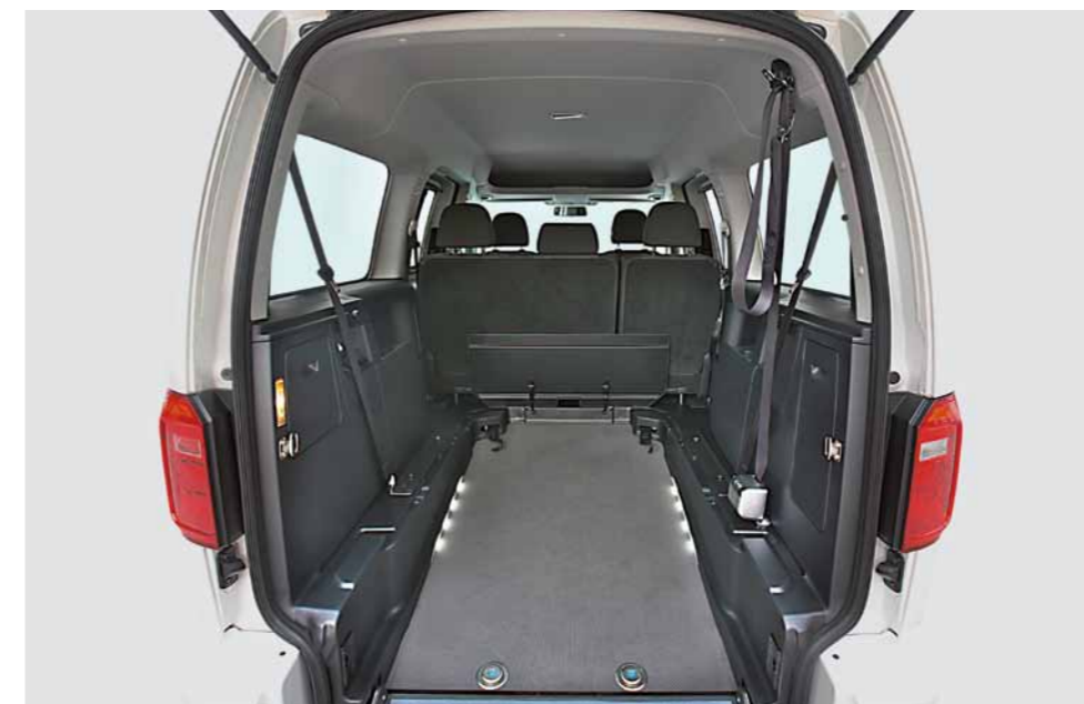
F-Style 3 Lowered Floor Conversion on Volkswagen Caddy Maxi
