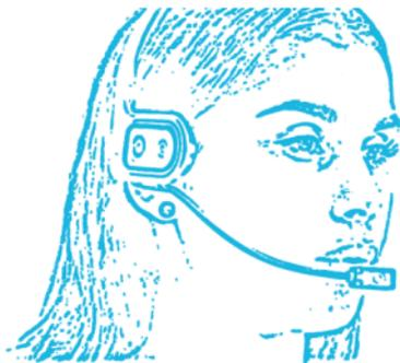
Testing the switch is simple. Puff into the sensor and a click is performed. Puff and keep puffing into the sensor and a long click (dragging) is performed as long as the puff continues.
