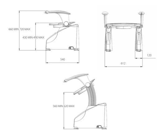
The vertical dimensions vary by 60mm due to adjustable feet.
